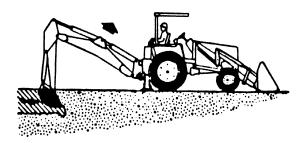
To obtain a cleaner trench and avoid the buildup of material directly in front of the backhoe, crowd out and completely curl the bucket while starting to lift it from the excavation. In this way, excess material will fall back into the excavation.
